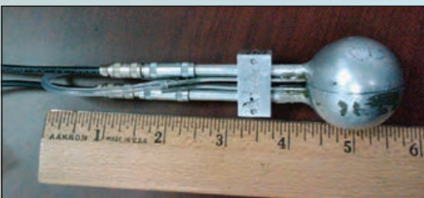
Figure 3. The third type of flux detector that will be assessed is a back-to-back (BTB) fission chamber, shown closed above right and open below.
