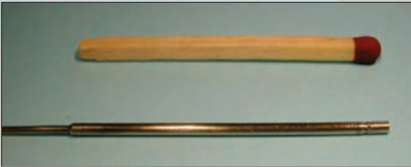
Figure 1. A sub-miniature fission chamber (bottom), a real-time state-of-the-art in-pile flux detection instrument developed by the Commissariat de Energie Atomique, is one of the flux detector technologies that will be assessed at the Advanced Test Reactor. A matchstick is shown as a basis for comparison.
