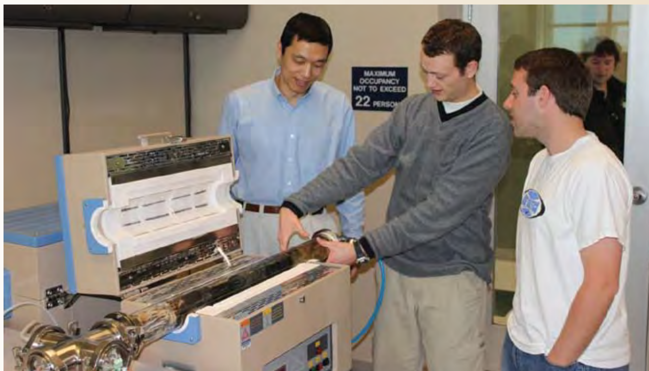
USU students and the principal investigator discuss the details of the thermal insulation arrangement in a thermal conductivity measurement system.
