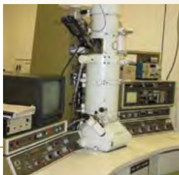
A JEOL 200CX TEM equipped with EDS and scanning system, and an electropolisher and dimpler at the Characterization Laboratory for Irradiated Materials, located on the UW campus in Madison, Wisconsin.
