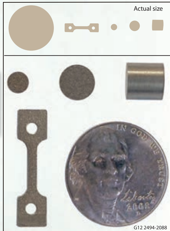
Figure 1. USU experiment material specimens.
