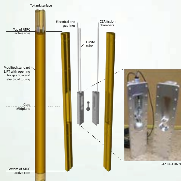
Figure 3. Fixture for positioning BTB and CEA miniature fission chambers in ATRC NW-LIPT.
