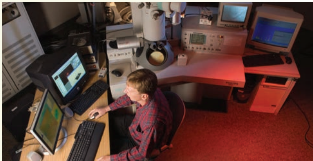
The high-resolution CM200 TEM with a new double-tilt holder for "hot" samples."
