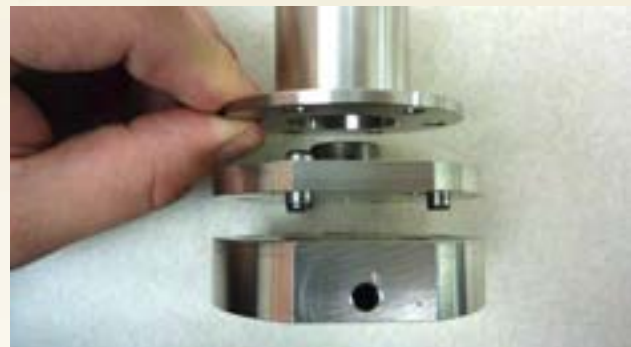
Figure 2. Side view of the shear punch fixture.
