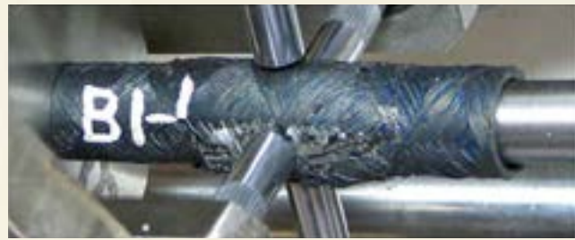
Figure 2. (top) Round 6 triplex tube undergoing mandrel-driven expanding plug burst testing.
