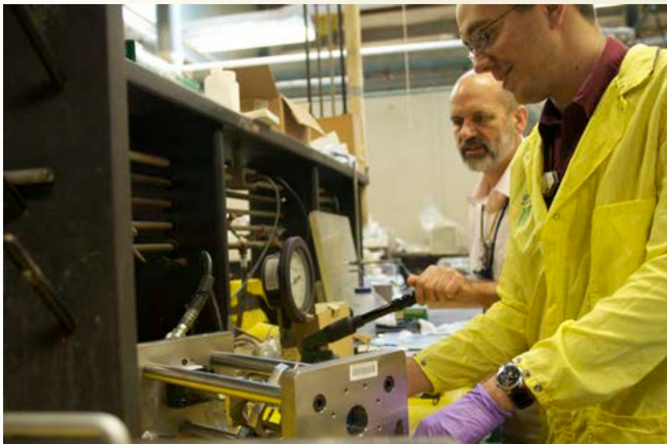
David Carpenter (bottom), and Gordon Kohse (top) removing SiC composite tube sample capsules from the irradiation rig in the reactor floor hot cell at the MITR.
