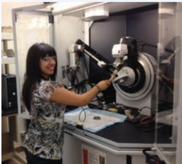
Research Assistant Ariana Alaniz using the high-resolution powder x-ray diffractometer.
