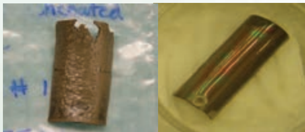
Figure 2. The bare tube (left) after two days in supercritical water at 500°C. The tube exhibited severe corrosion and swelling, and the original shape had changed. The cladding tube with TiN coating (right) showed no change in shape after the two day test. The surface color had changed slightly, but there was no obvious degradation to the tube itself. These results clearly demonstrate the effectiveness of the coatings.
