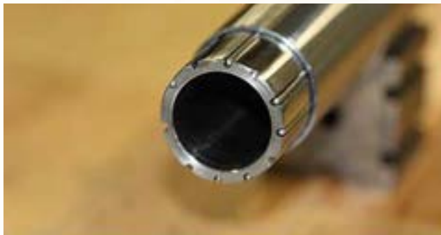
Figure 2. The thermocouple and gas feed assembly.
