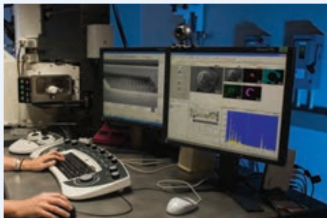
The focused ion beam produces sharp, clear images of 3-dimensional 20um cubes of materials.
