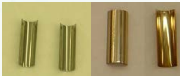
Figure 1. Polished cladding tubes without coating (left) and cladding tubes with TiN coating on the front and back (right).
