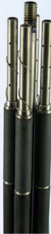
Tubes of the new ceramic composite material are loaded into a capsule and irradiated in the MIT reactor. These specimens are subjected to the same conditions found inside the core of a full-sized power reactor.
