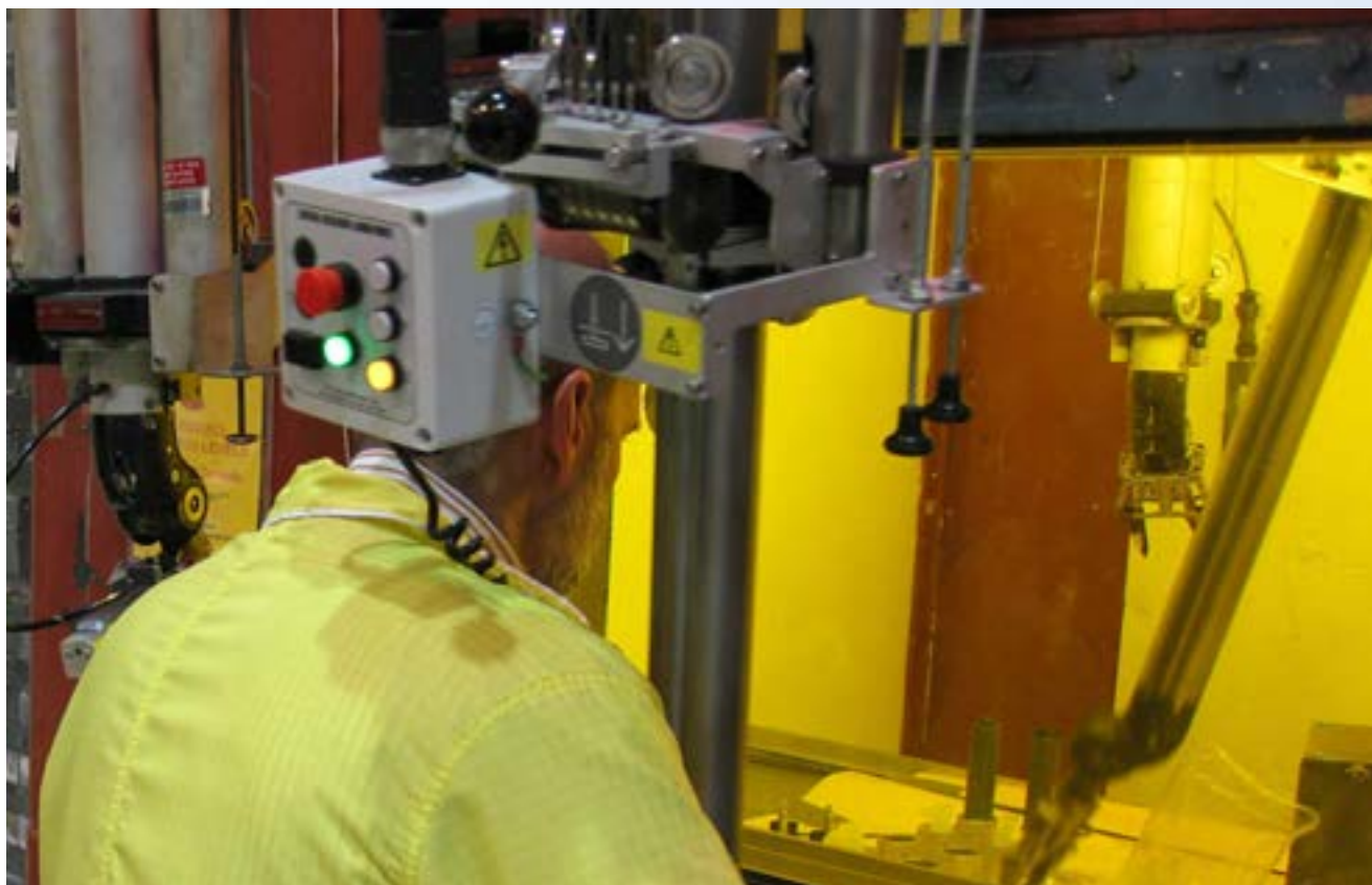
Research engineer Gordon Kohse unloads a ceramic composite irradiation capsule inside a hot cell at the MIT reactor.
