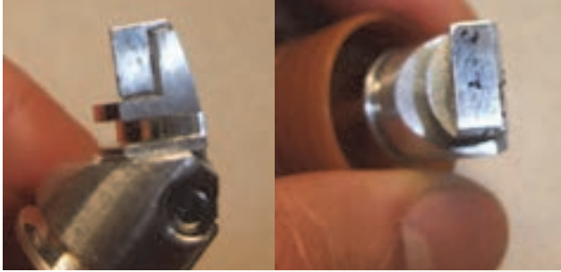
Figure 2. Modified fixture used for the EBSD analysis.
