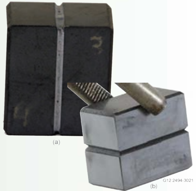
Figure 2. (a) An SiC bond block specimen EWIP4-1 before, and (b) after irradiation in the MITR water loop.
