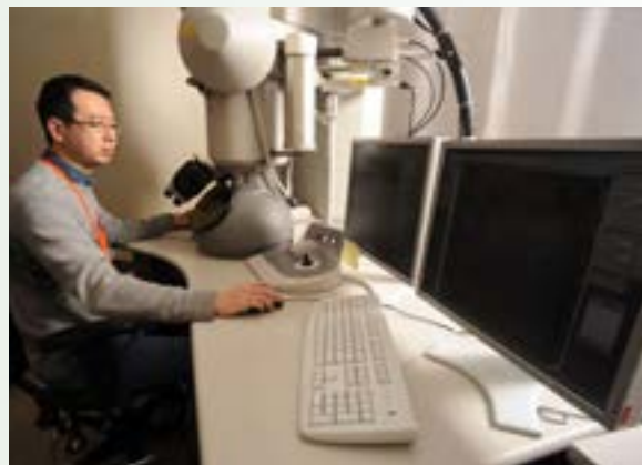
Transmission electron microscope, one of many PIE capabilities in the Microscopy & Characterization Suite (MaCS) at the Center for Advanced Energy Studies in Idaho Falls, Idaho.
