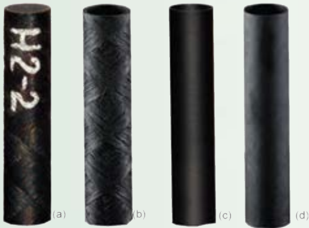
Figure 1. (A Triplex SiC tube specimen (a and b) and a monolithic SiC tube specimen (c and d) before and after irradiation in the MITR water loop (> 800 effective full-power days exposure).
