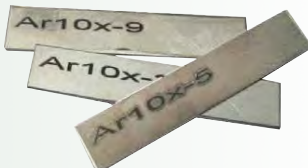
Figure 2. Zirconium specimens used for irradiation and post-irradiation examination.
