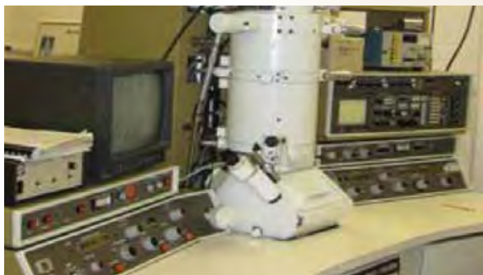
A JEOL 200CX TEM equipped with EDS and scanning system, and an electro-polisher and dimpler at the Characterization Laboratory for Irradiated Materials, located on the UW campus in Madison, Wisconsin.
