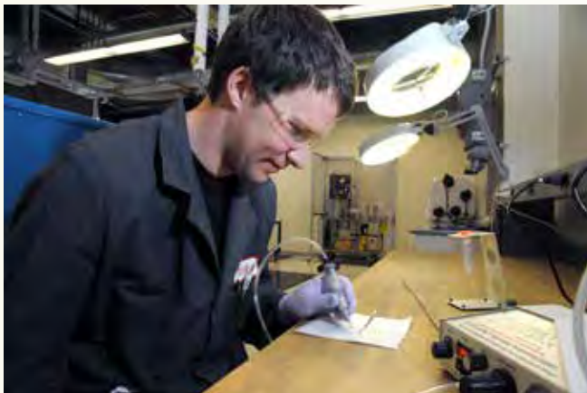
Research scientist Troy Unruh injects epoxy onto specialized micro-pocket fission detector (MPFD) components. These detectors are used to simultaneously measure thermal neutron flux, fast neutron flux and temperature.
