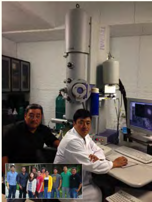
Dr. Yongho Sohn and his University of Central Florida research group are characterizing metallic fuels and materials, which are potential candidates for advanced reactors, to understand the specific effects of high temperatures and irradiation. Here, Sohn (left) and doctoral candidate Youngjoo Park use a transmission electron microscope to examine samples. The full research group (inset photo) includes students and scholars in front of Sohn's Laboratory for Materials and Coatings for Extreme Environment. Photos provided by Yongho Sohn's research group.
