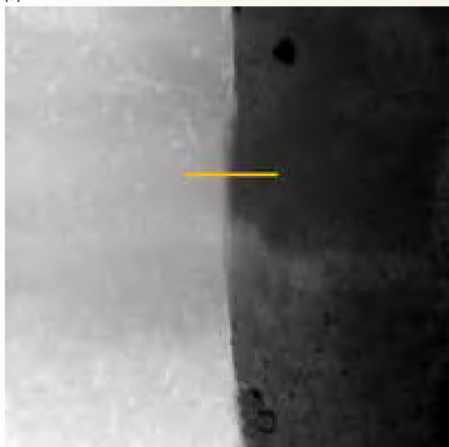
Figure 1. STEM images and EDS elemental line scans of the \text{TiO}_2 and \text{Y}_2\text{O}_3 samples irradiated with 5 MeV Ni ions at 500° C for:
