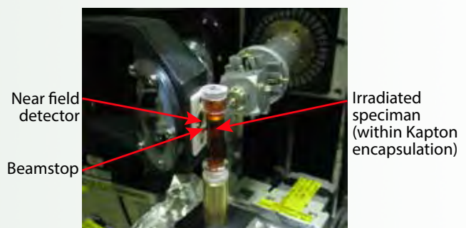
Figure 1. Specimen and detector configuration for HEDM measurements.
