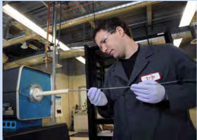
Research scientist Troy Unruh, shown here inserting an MPFD prototype into the HTTL furnace for heating evaluations, is pursuing his doctorate from ISU.
