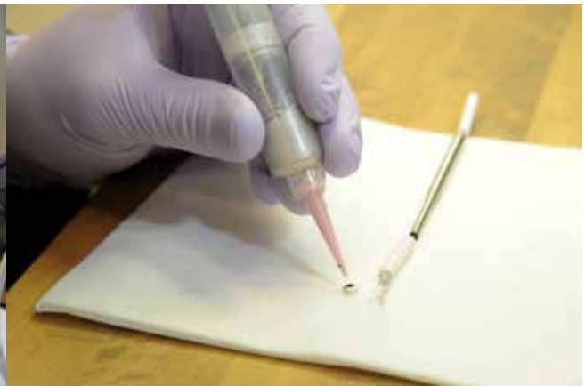
Research scientist Troy Unruh injects epoxy onto specialized micro-pocket fission detector (MPFD) components. These detectors are used to simultaneously measure thermal neutron flux, fast neutron flux and temperature.
