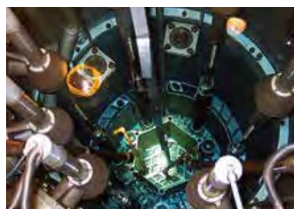
Annular fuel rig in the MITR core.
