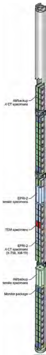
Figure 4. Typical irradiation test train containing CT, tensile, and TEM specimens.
