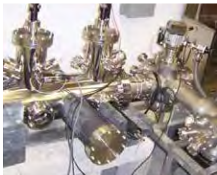
The Positronium Annihilation Lifetime Spectrometer, located in the PULSTAR reactor facility on the NC State North Campus in Raleigh, N.C.
