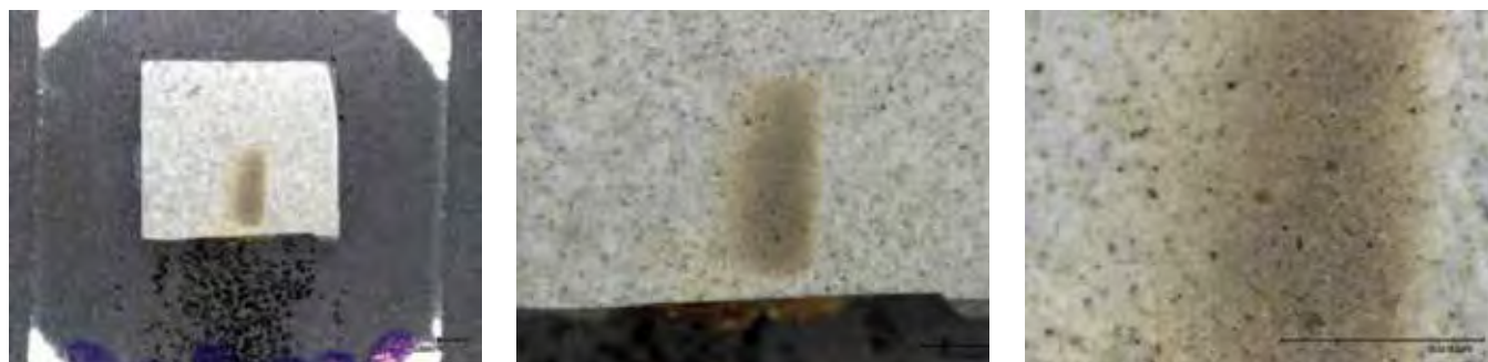
Figure 1. Optical microscope image at 50, 100, and 150 \times magnification shows discoloration and cracking in the nanoconcrete surface. This flux used in this irradiation was 5 \times 10^{13} protons/cm 2 and resulted in significant volatilization from the surface.
