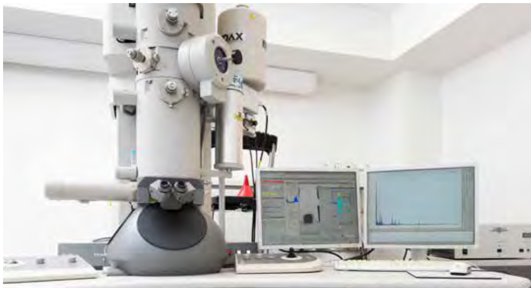
Dual Beam Focused Ion Beam (FIB) and Scanning Electron Microscope (SEM) at the Nuclear Fuels and Materials Characterization Facility, University of Florida (Courtesy of University of Florida).
