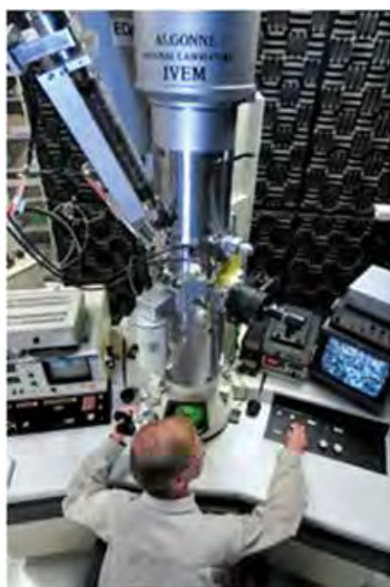
Figure 1. (Left) Argonne-IVEM for in situ TEM observation of \text{UO}_2 irradiated with 300 eV Xe. (Right) SRIM calculation showing the radiation damage level (dpa) and Xe concentration at 5 \times 10^{16} ions/cm 2 .
