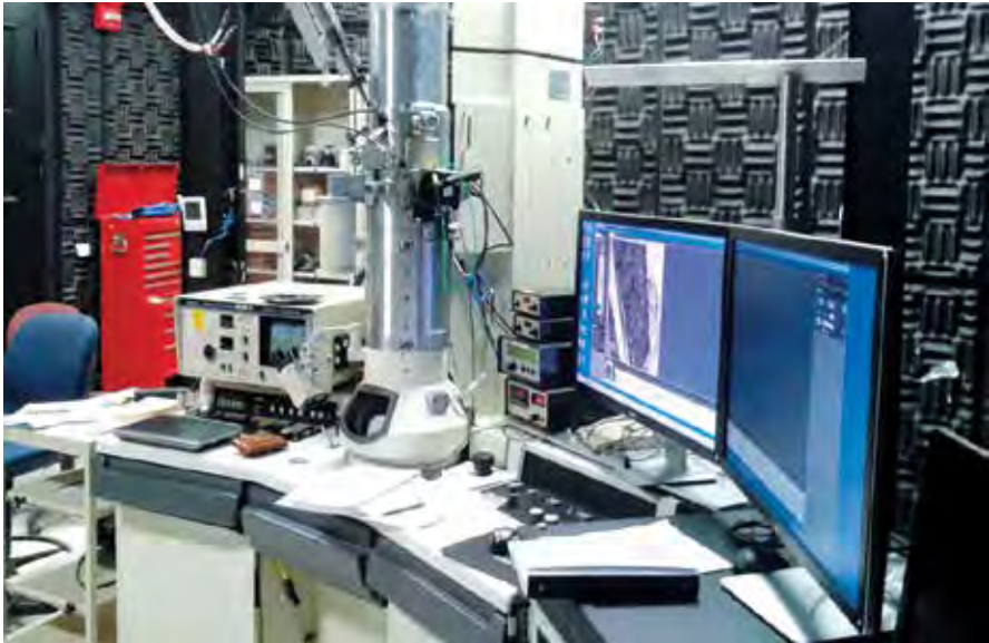
Figure 5. Picture of the ANL IVEM in use during in situ ion irradiation experiment.
