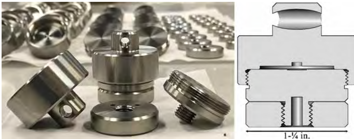
Figure 3. (Left) Photograph and (right) cross-sectional schematic of updated three-piece sample holder design for polishing small irradiated samples in hoods, shielded storage, and secure transferring of samples between hoods and instruments.
