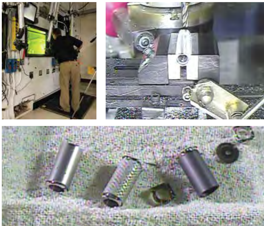
Figure 3. Disassembly of Fire Rabbit at the Irradiated Materials Examination and Testing Laboratory following neutron irradiation in the High Flux Isotope Reactor. Top left: a hot-cell operator opening the capsule; top right: capsule housing being carefully milled to retrieve the delicate samples; bottom: retrieved specimens with aluminum thermal homogenizer jacket (left), SiC/SiC composite tube with centering thimbles (middle), and monolithic SiC tube (right).
