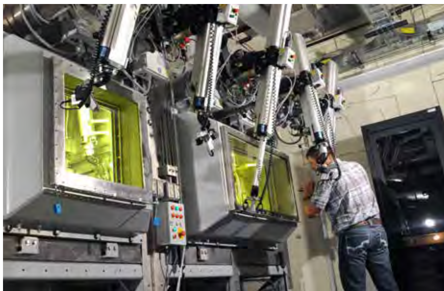
Hot cells housing INL's Irradiation Assisted Stress Corrosion Cracking instrumentation
