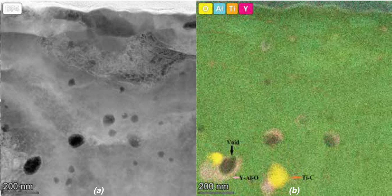
Figure 1. (a) High-angle annular dark-field imaging and (b) composition map (O-Al-Y-Ti) of the stir zone of friction stir welded MA956 irradiated with 5 MeV Fe++ at 450°C up to 200 dpa.
