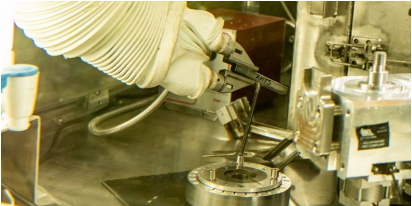
Tensile samples are loaded onto the AMTS cartridge for measuring mechanical properties.
