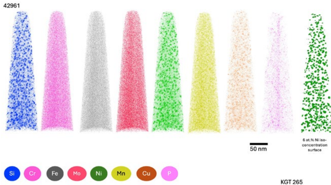
Figure 2. APT reconstruction data from neutron-irradiated HT-9 ORNL heat (KGT 265, 469°C, ~4 dpa).
