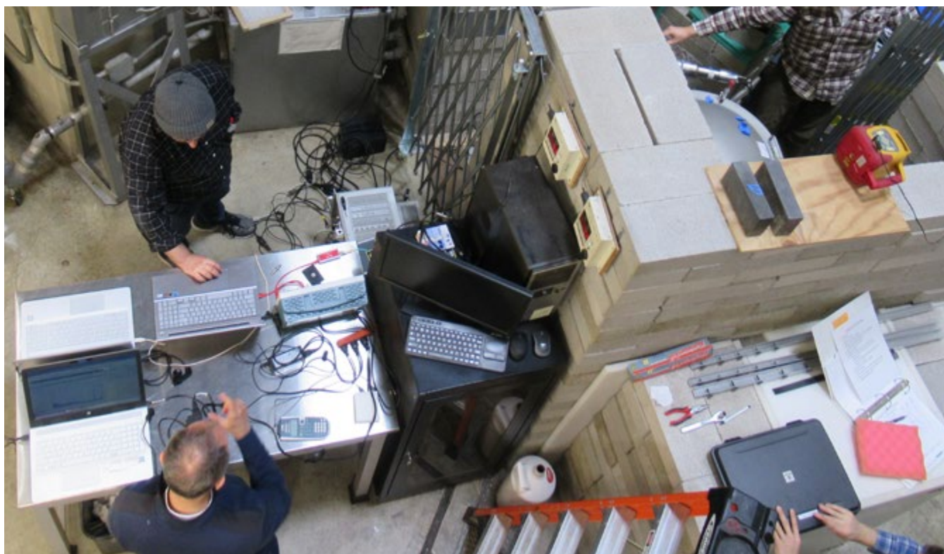
(Top left) University of Michigan doctoral student Alexander Kavner calibrates the germanium detector placed in the thermal neutron beam and the tagging sodium iodide detector. (Bottom left) PI Igor Jovanovic reviews the in-situ data from testing. Irradiations for Jovanovic's RTE, "Measurement of 254-eV Nuclear Recoils in Germanium" were performed at The Ohio State University Research Reactor using the Thermal Neutron Beam Facility.
